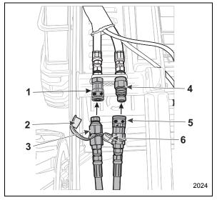
Figure 3-30 Auxiliary Hydraulic Quick Connects
